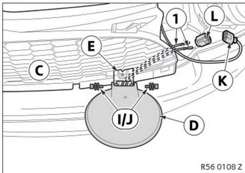
Step 6: Connect the adapters of the LED daytime running lamps to the wiring harness.
