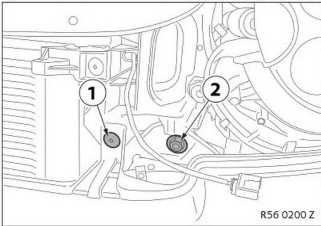
Step 3: Secure the bracket using nuts and bolts. Repeat on the other side.
